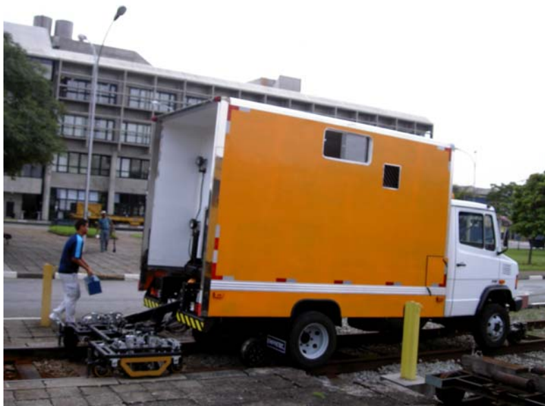
Fig. 7. Testing equipment hanged on the modified truck.
